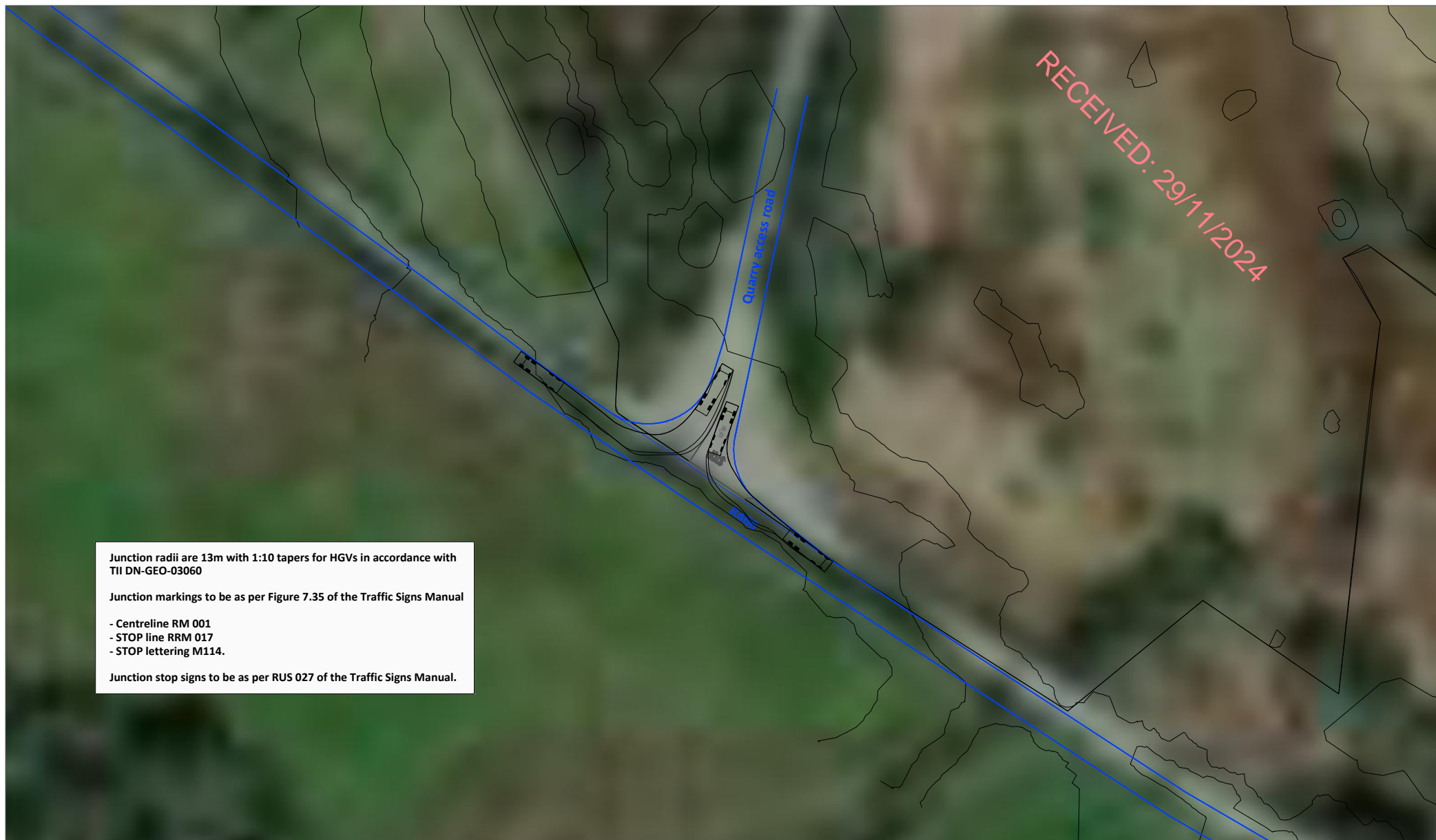
Figure A13-2-3 Quarry access junction on R466 - Autotrack assessment for large tipper truck (2.5m x 10.2m)
